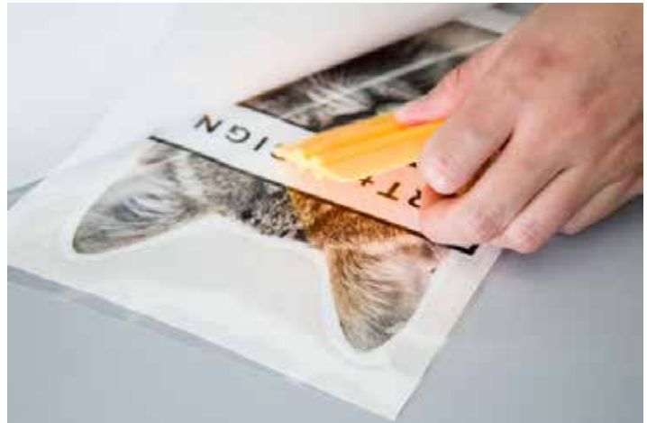
Fig 6 - Apply (clear) application tape on printed vinyl
