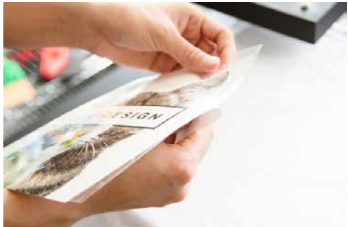
Fig 7 - Removing the release liner (backing)
