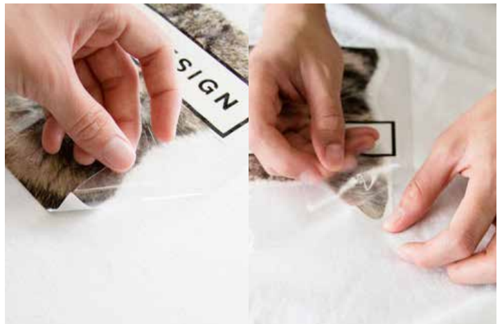
Fig 11 - Peeling transfer tape. Not fully adhered (left) and fully adhered (right)
